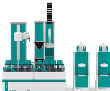
**Figure 6.** Metrohm offers solutions for the automated titration of the residual alkali content in cathode materials. This system is equipped with the Dis-Cover functionality to prevent the uptake of  $\text{CO}_2$  from the environment. Before the titration, the system automatically removes the cover for the most accurate results.
