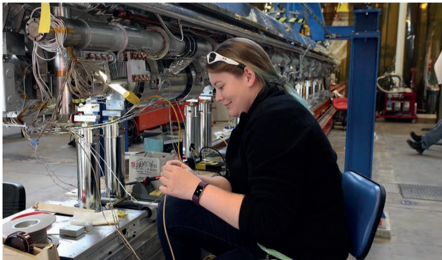
Jefferson Lab cryomodule construction and testing. Linked together and chilled to nearly absolute zero, 37 of these cryomodules will accelerate electrons to almost the speed of light. (Credit: Fermi National Accelerator Laboratory)
