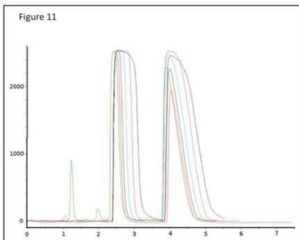
11. Extraction-injection of warfarin; overlays of chromatograms from 8, 12, 20, 30 and 40 ml injected from an extractor (50 x 10 mm) packed with 400 mg warfarin coated on 2 g Daiso C-1 (50  $\mu$ m). Column: CHIRALCEL OD-H 150 x 21.2 mm. Mobile phase 20% methanol in CO<sub>2</sub> at 60 ml/min flow rate, 40°C, back pressure 100 bar.
