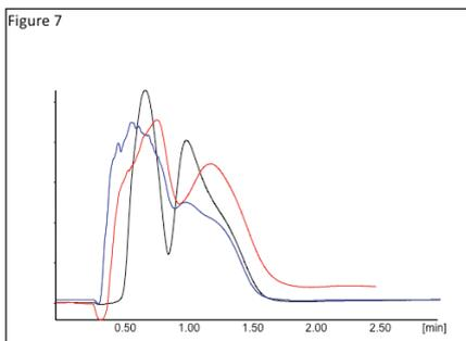
7. Overlays of chromatograms of 300 mg guaiphenesin in methanol (150 g/l, 2 ml, black line), in 20% hexane-alcohol (22.4 g/l, 13.4 ml, red line) and in pure ethanol (22.4g/l, 13.4 ml, black line). Conditions as Figure 5.
