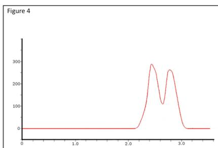
4. Analytical separation of trans-stilbene oxide (TSO) enantiomers by mixed stream and modifier stream injections. Sample TSO, 5 g/l, injection volume 2 ml. Column: CHIRALPAK IA 250 x 21.2 mm. Mobile phase 15% methanol in  $\text{CO}_2$  at 100 ml/min flow rate, 40°C, back pressure 100 bar.
