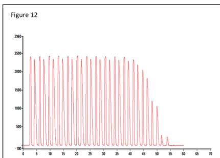
12. Stacked injection separation of warfarin enantiomers. 760 mg warfarin coated on 2 g Daiso C-1 (50  $\mu$ m) packed into an extractor (100 x 10 mm) with 30 second injection time. Conditions as for Figure 11. Separation time 6.3 minutes, cycle time 3.5 minutes.
