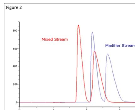
2. Preparative separation of guaiphenesin enantiomers by mixed stream and modifier stream injections. Sample 100 g/l, injection volume 390  $\mu$ l. Conditions as Figure 1.
