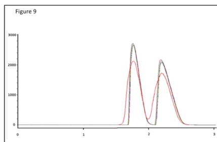
9. Overlays of chromatograms of 52 mg TSO in methanol (52 g/l, 1 ml, red line) and 4 consecutive injections of 1 second (= 1 ml) from 2 g of TSO in an extractor 100 x 10 mm. Conditions as Figure 1.0°C, back pressure 150 bar.
