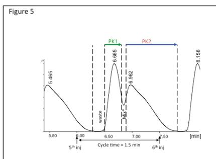
5. Preparative separation of guaiphenesin enantiomers by mixed stream injection. Sample 150 g/l, injection volume 2.7 ml. Column: CHIRALCEL OD 20 $\mu\text{m}$ , 250 x 21.2 mm. Mobile phase 20% ethanol in  $\text{CO}_2$  at 180 g/min flow rate, 0°C, back pressure 150 bar.
