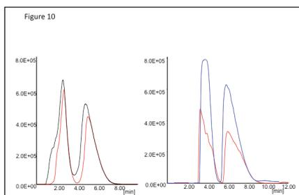
10. Separations of warfarin enantiomers. (a) overlays of 90 (6 ml) and 135 mg (9 ml) of warfarin in ethanol @ 15 g/l and (b) 90 and 150 mg warfarin from extraction injection. Column: CHIRALCEL OD 20  $\mu$ m, 250 x 21.2 mm. Mobile phase 20% ethanol in CO<sub>2</sub> at 100 g/min flow rate, 25°C, back pressure 105 bar.
