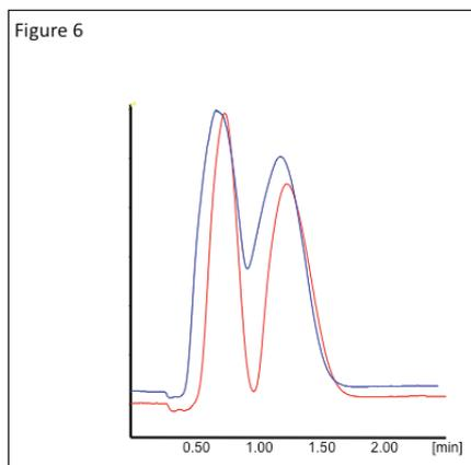
6. Overlays of chromatograms of 112 mg guaiphenesin using mixed stream injection (5 ml) and samples dissolved in 20% ethanol in hexane (red line) and 100% ethanol (blue line). Conditions as Figure 5.
