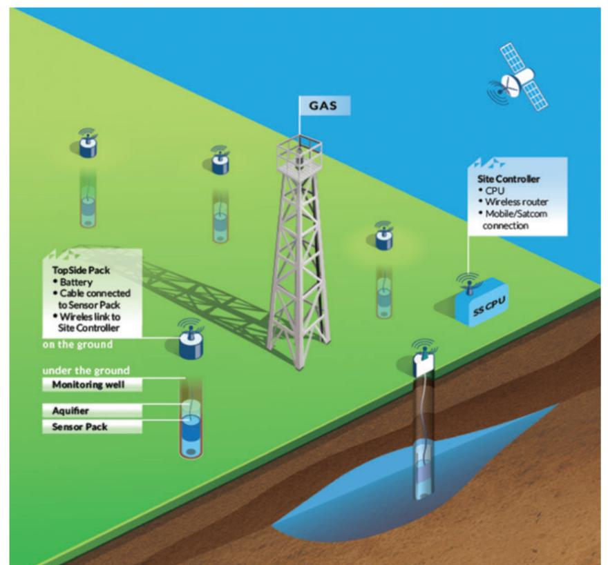
Figure 1: visualisation of ShaleSafe technology deployed in the vicinity of a shale gas well site.
