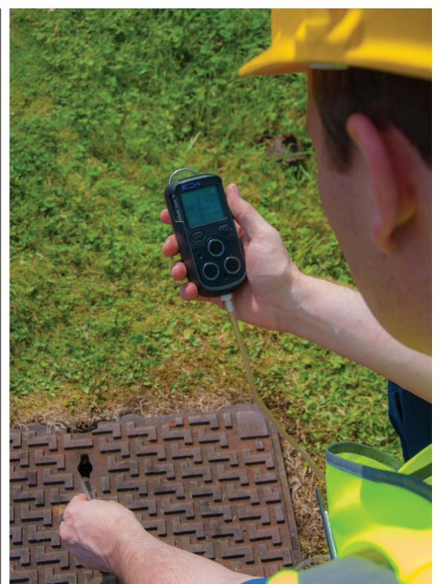
Pumped sample collection using PS200 hand-held gas detector
