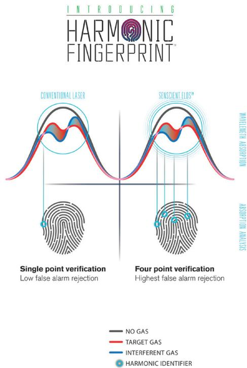
Fig 3. Senscient ELDS Harmonic Fingerprint Theory of Operation
