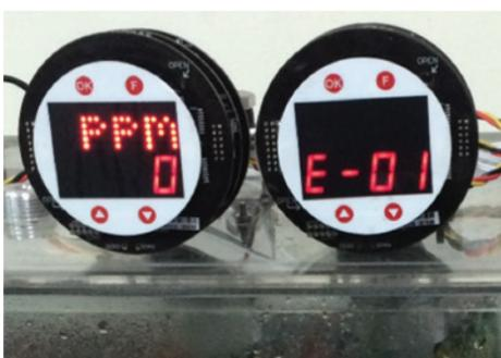
Figure 5: Fixed PIDs a) with (left) and b) without (right) condensation control
