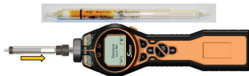
Figure 7: Pre-filter tube attached to PID for specific benzene measurements in a portable instrument.
