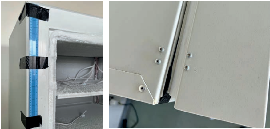
Figure 5: Left; securing the 45cm long ruler to the top left-hand side of the opened freezer created at 3.8mm gap (right) between the door seal and the freezer chamber. The obstructed seal spanned the entire height of the top freezer compartment (1) and ~50% of that of compartment 2.
