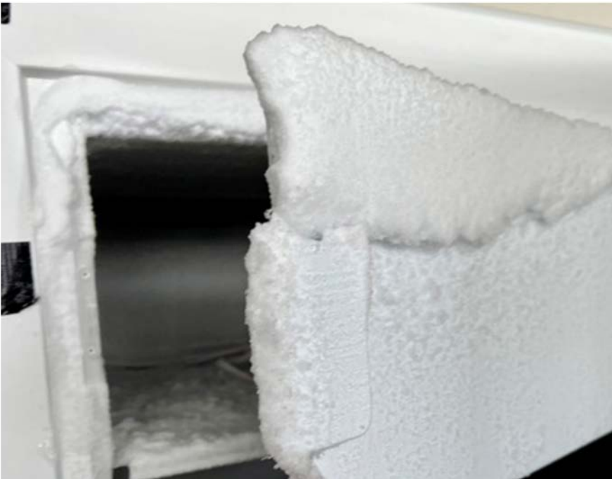
Figure 12: Icing build up progressed throughout the testing steps when the door seal was obstructed and was localised to the inner door and door frame of compartments 1 and 2.
