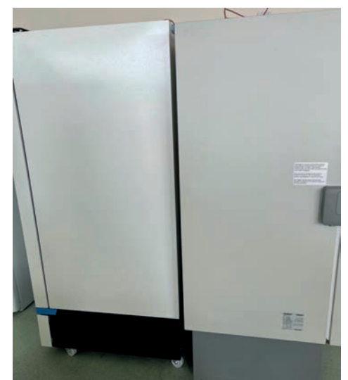
Figure 4: On the left, poor spacing. Placing a ULT freezer back to back with another is another form of poor spacing was examined separately.
