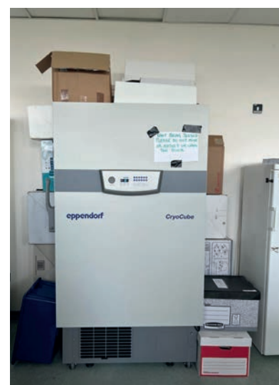
Figure 4: On the left, poor spacing. Placing a ULT freezer back to back with another is another form of poor spacing was examined separately.
