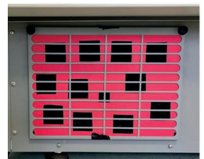
Figure 3: The filter with 75% of the surface area blocked.
