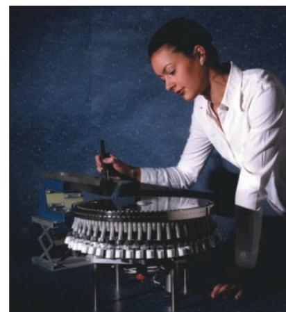
Figure 1. A 100 stage spinning riffler for precision sample splitting.
