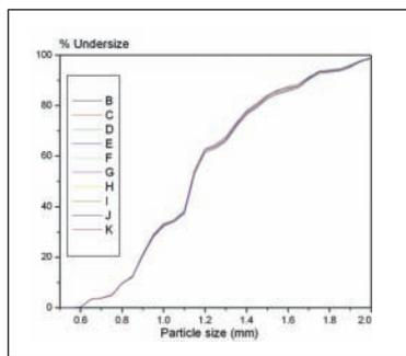
Figure 3. Repeatability measurement on 10 x 20g samples (Haver CPA).
