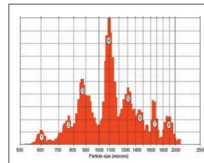
Figure 2. Individual peaks in a multimodal image analysis standard.
