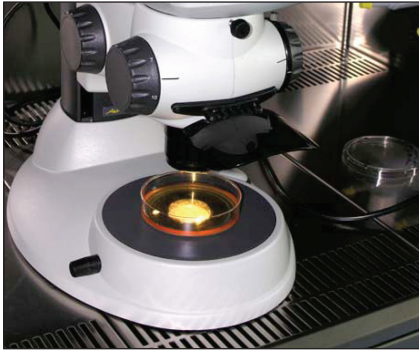
Figure 2. Shows the substage of the Lynx with tilting mirror and the pseudo brightfield and darkfield effect.
