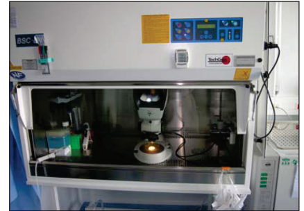
Figure 1. Vision Engineering's patented Dynascope® head is the key feature of the Lynx, allowing the system to deliver optimum clarity.
