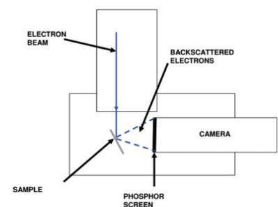
Figure 2. Schematic of EBSD setup
