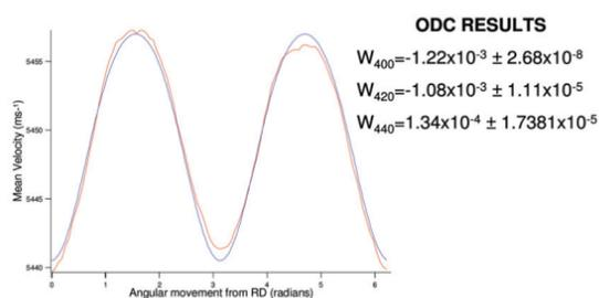
Figure 4. Ultrasonic Velocity vs. angle subtended from the rolling direction over a 360 degree rotation. The red trace is the ultrasound data, the blue trace is the solution to Eqn 3.
