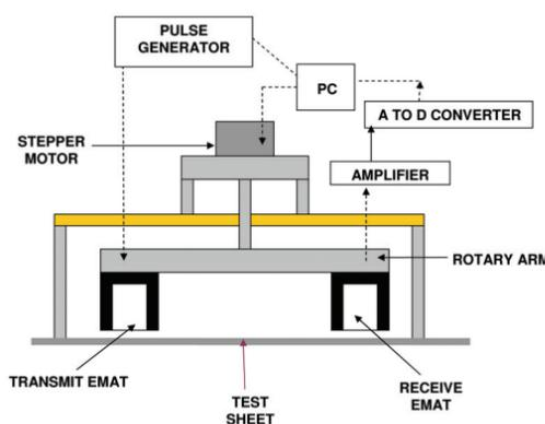
Figure 1. Schematic of EMAT-EMAT system setup
