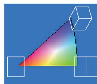
Figure 3. EBSD Inverse Pole Figure (IPF): indicates the colour distribution for all crystallographic orientations
