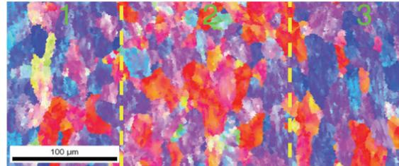
Figure 5. 1<sub>11</sub> EBSD scan taken from AL104232. The left and right hand side are below the RD-TD plane surfaces. [111] orientation dominant in layers 1 and 3.
