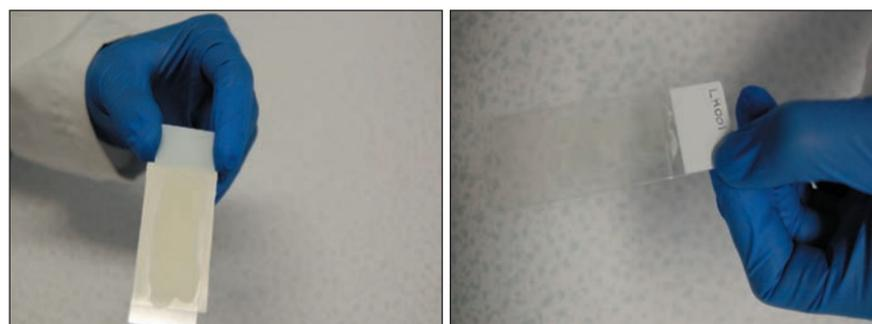
Figure 3. The Easylift coated slide. This image shows the slide viewed from the uncoated side, with the protective paper backing film on the underside of the transparent coating material.
