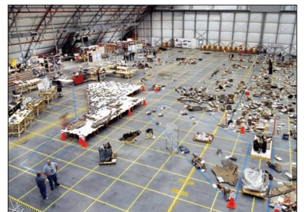
Figure 4. Reconstruction of the Columbia debris at the Kennedy Space Center
