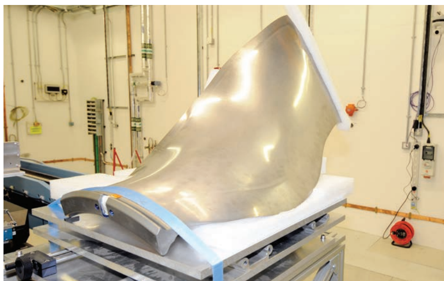
Fan blade from Rolls-Royce engine on the JEEP beamline, I12.
