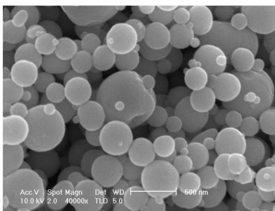
Figure 1. Scanning Electron Micrograph of PZT (lead zirconate titanate)
