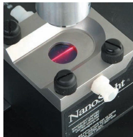
Figure 1. Picture of laser module showing beam passing through sample and viewed from above via microscope objective.
