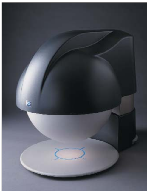
Figure 1. VideometerLab 2. Up to 20 wavelengths via LEDs, uniformly spaced around the inside of the integrating sphere are strobed successively each generating a monochrome image.
