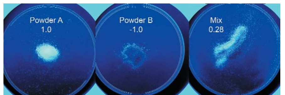
Figure 13. Each component within the mixing process is assigned a weighting based on its spectral profile. The 'Mix' value indicates to the operator the make-up of the sample from 'Powder A' and 'Powder B'.
