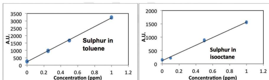
Figure 1: Total sulphur content in different organic solvents at concentration values below 1ppm.
