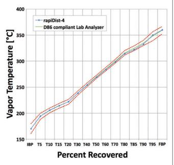
Figure 3: Outstanding reproducibility and correlation of the rapiDist-4 with an ASTM D86 compliant laboratory analyzer. Reproducibility limits according to ASTM D86 are marked as dotted lines.
