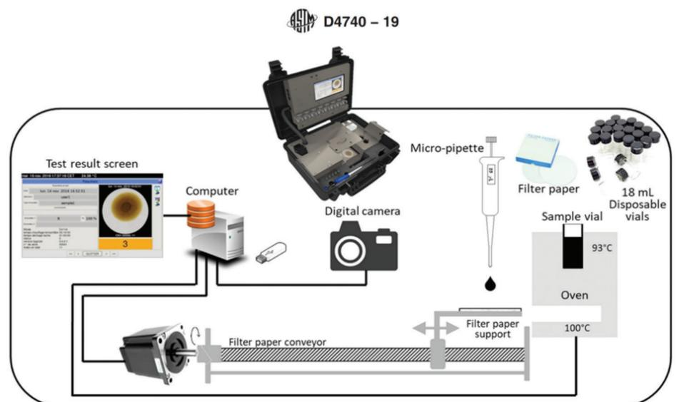
Figure 2. Schematics of the automated apparatus (Source : ASTM [1])
