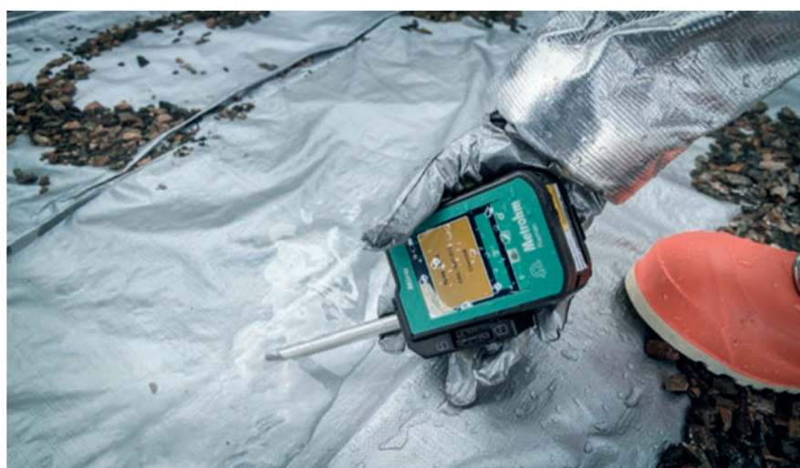
Figure 2. With the ball probe attachment, substances can be measured in direct contact with the probe, meaning that the user no longer has to maintain a certain distance.
