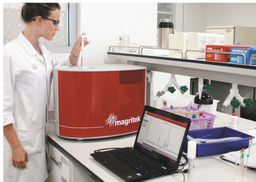
An operator places a standard NMR sample tube inside the Spinsolve benchtop NMR system
