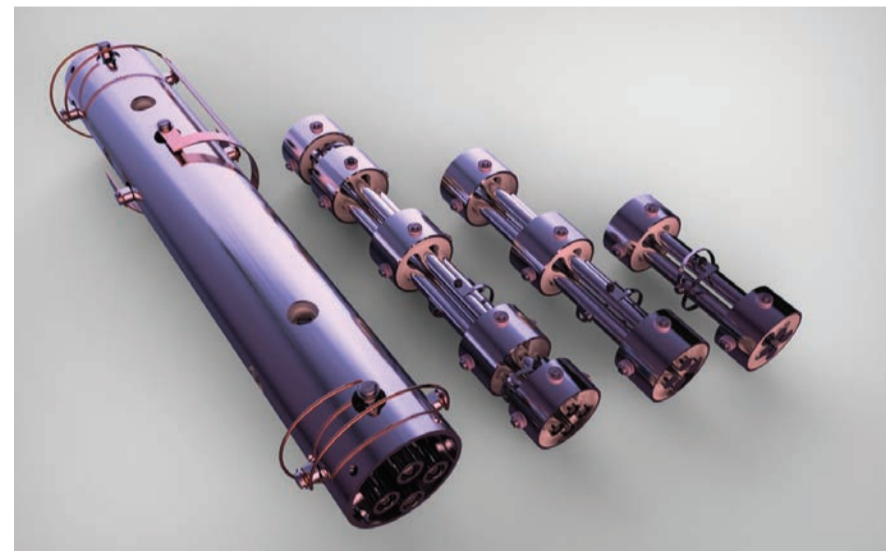
Figure 3: Quadrupole mass filters shown, from 20mm pole diameter to 6mm pole diameter offer mass range options up to 5000u. 200u mass range is typically used for most real time gas analysis applications.
