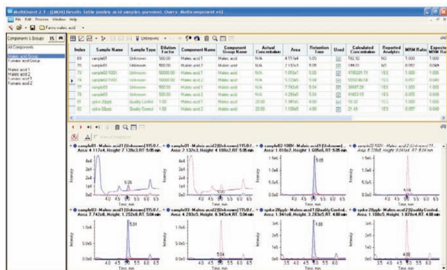
Figure 4. Results for maleic acid in different food samples, the 'Multicomponent' query in MultiQuant™ software was used to identify target analytes based on their MRM ratio
