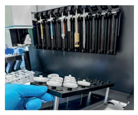
The patented rotating foot provides operational advantages, enabling automated tool changes for analytical syringes, SPE cartridges,  $\mu$ SPEed syringes, syringe disc filters, controlled piercing of septa-sealed vials, as well as precise aspirating and dispensing. Its capabilities are further enhanced by features such as a wash station, an optional large volume dispenser, and an optional direct injection port.
