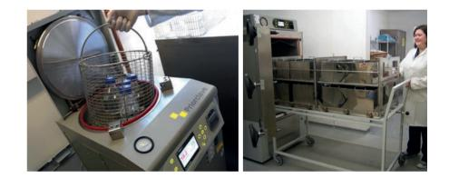
Laboratories looking to invest in a new autoclave and requiring a higher throughput may initially look to purchase a rectangular chamber design. Size for size in chamber capacity, it would seem to offer better loading than that of a cylindrical machine and look to be the right choice; more items could be crammed into the chamber. Are they a better buy? Is it false economy?
