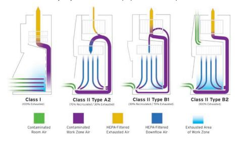
There are three classes of BSCs that offer varying levels and types of protection [1, 5, 6]. Class I cabinets protect personnel and the environment but do not provide HEPA-filtered air to the work zone for the product's protection [1, 5, 6]. If your risk assessment identifies a need to protect the product from external contaminants, you may need to select a Class II or Class III biological safety cabinet.
