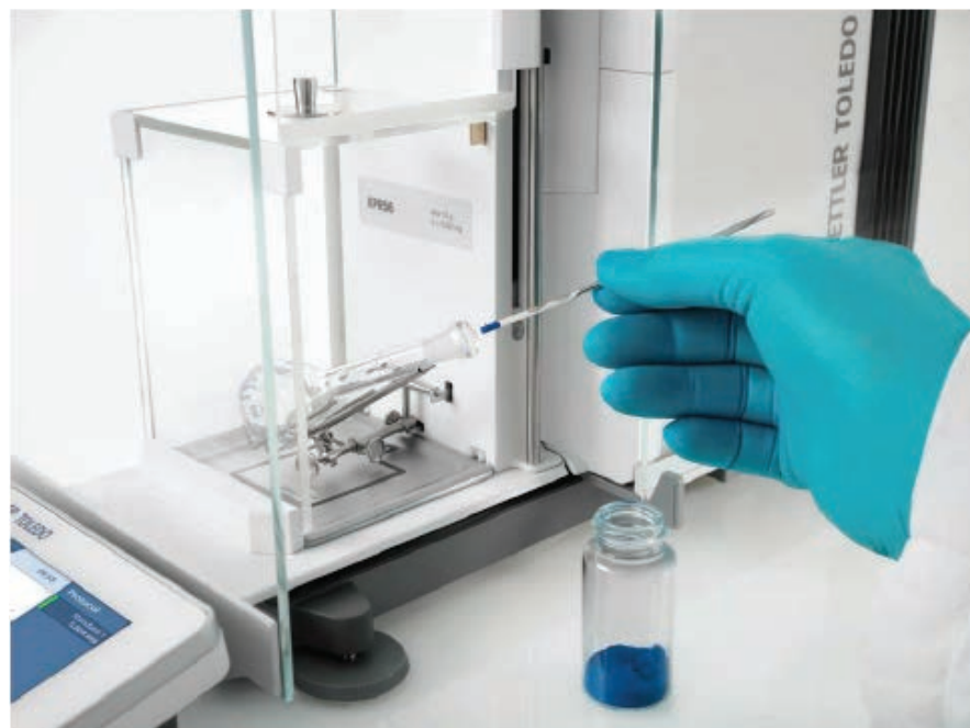
Figure 5: ErgoClip holders stabilise the tare container in the XPR and XSR analytical balance to enable one-step direct dosing and eliminate sample-transfer errors and scattering.
