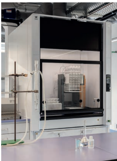
Figure 1: Saving energy by closing the front sash of the fume cupboard.
