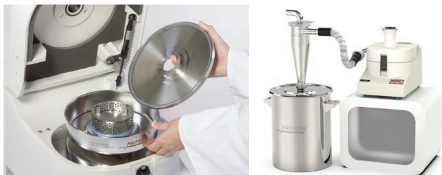
Figure 1: Inside of a Variable Speed Rotor Mill PULVERISETTE 14 classic line, showing fixed collection vessel, rotor and sieve ring. The stainless steel Cyclone separator is shown on the right.
