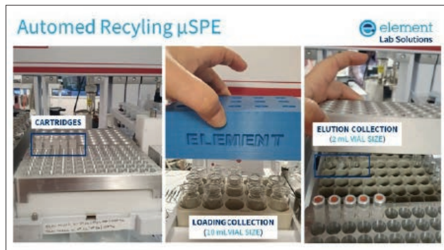
Figure 2: Customised recycling station for the automated miniaturised SPE of derivatised sterols in plasma
