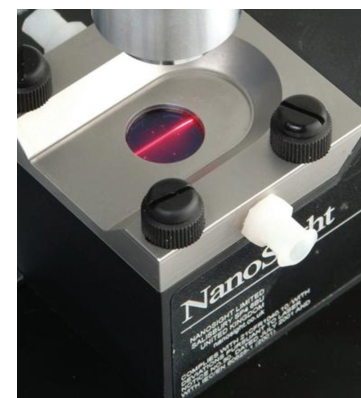
Figure 1. A specially designed flow cell.
