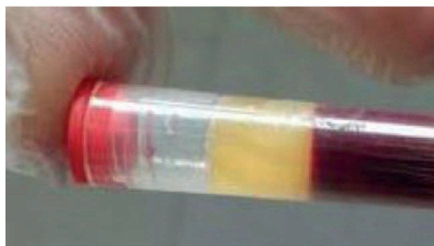
Figure 11: Ice plug forming at the top of the sample, leading to tube damage
