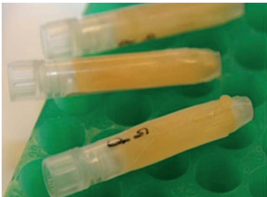
Figure 8: Fill error of 5% leads to the tube cracking
