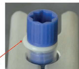
Figure 4: The expansion of the sample in the tube can lead to the cap or O ring 'popping out'.
