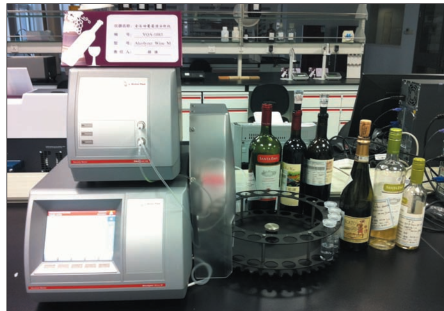
Figure 2. Instrument combination for wine analysis. DMA 4500 ME, Alcolyzer Wine M and Xsample 122
