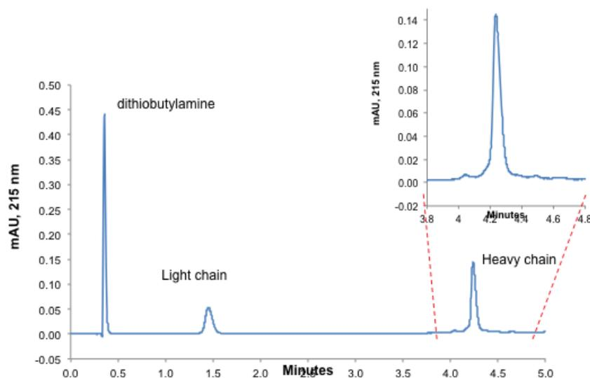
Figure 5: Resolution of SigmaMAb subunits on BIOshell A400 Protein C4w
