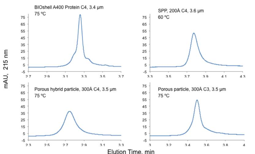
Figure 3: Column Performance comparison with SigmaMAb at optimal temperature
