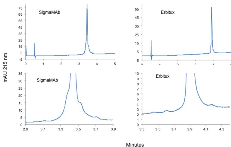
Figure 2: Fast Chromatography of intact monoclonal antibodies on BIOshell A400 Protein C4
