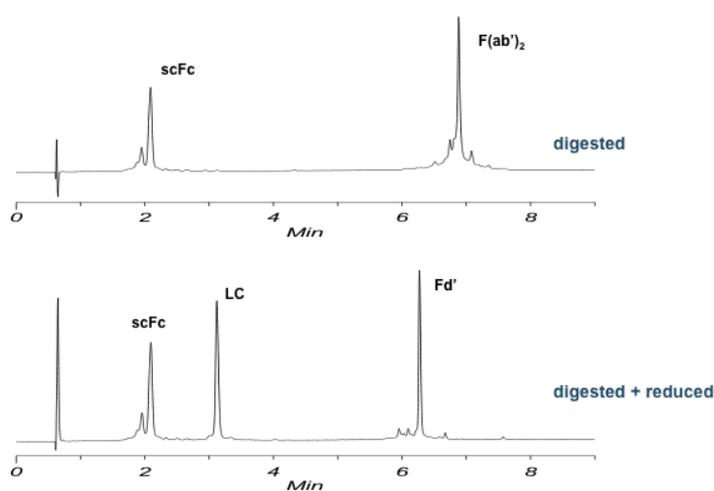
Figure 4: Resolution of IdeS fragments of SigmaMAb (p/n MSQC4) on BIOshell A400 Protein C4, before and after reduction
