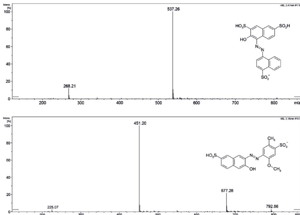
Figure 3: MS spectra of the two colorants Amaranth ( $[M-3Na^+ + 2H^+]^+$ ,  $m/z = 537.3$ , top) and Allura Red AC ( $[M-2Na^+ + H^+]^+$ ,  $m/z = 451.2$ , bottom) eluting at 2.47 and 3.18 minutes, respectively. For MS conditions see Figure 2.
