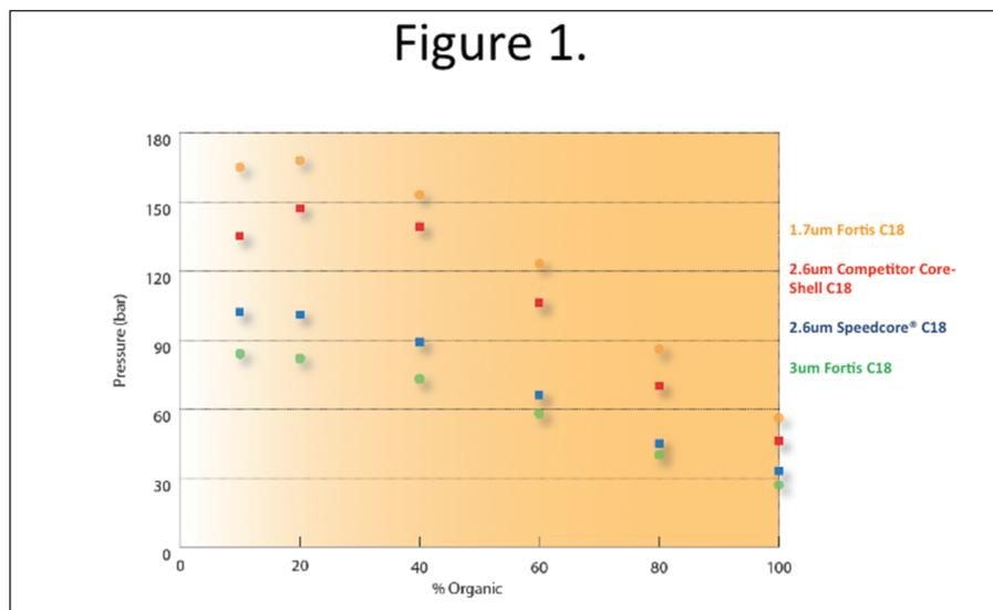
Figure 1. (Backpressure of 2 commercial core-shells vs fully porous particles)
