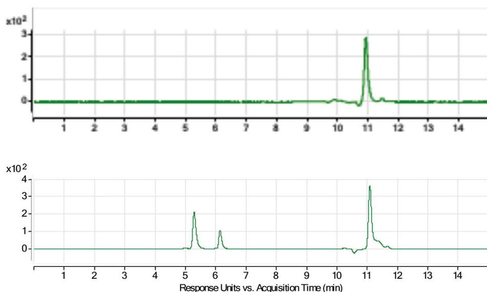
Figure 1: Irreversible adsorption occurring on a prototype SEC column, compared to final column. The three main peaks relate to Fab, Fc fragments of an IgG protein and the solvent peak. It is very evident that the peaks are not eluting due to adsorption issues.
