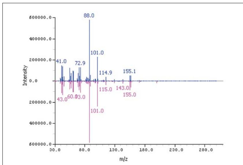
Figure 7: Decanoic acid, ethyl ester at 22.228, 1.017 89% match
