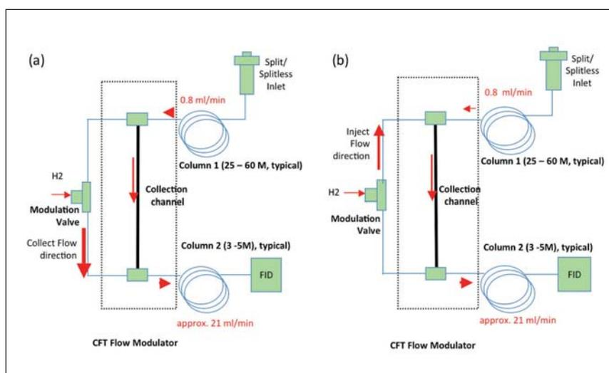
Figure 2: Agilent Capillary Flow Modulator. (a) Load Position; (b) Inject position
