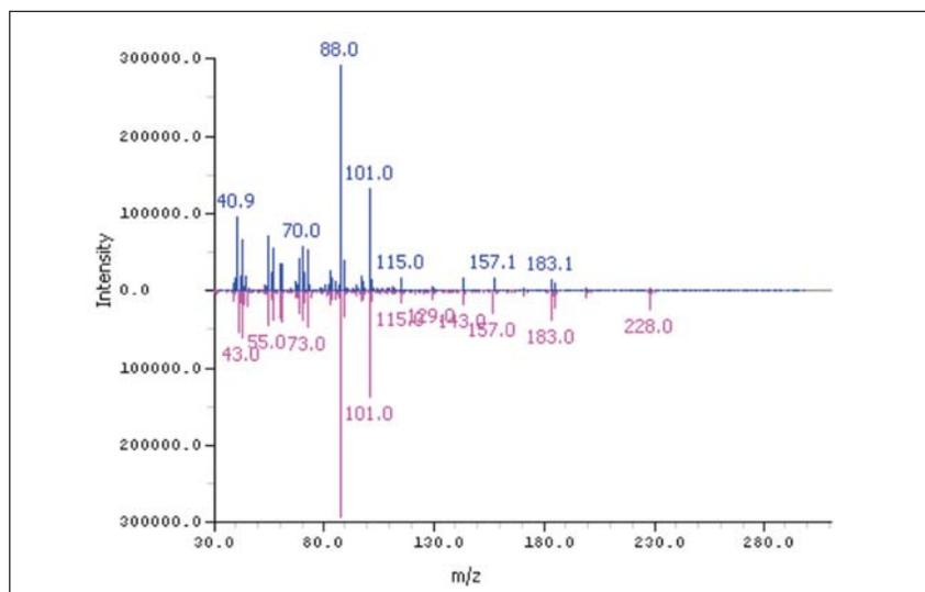
Figure 8: Dodecanoic acid, ethyl ester at 26.955, 1.081 85% match
