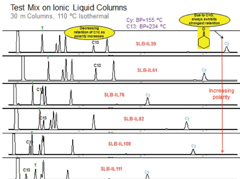
Figure 3: Comparison of the Ionic liquid Column Selectivity, 30m x 0.25mm ID x 0.25µm df, Oven: 110°C, Inj. 250°C, Det. FID 250°C, Carrier Gas: Helium, 25cm/sec at 110°C, Injection: 1µl, 100:1 Split, Sample Components: toluene, ethylbenzene, p-xylene, isopropylbenzene, cyclohexanone, 1,2,4-trimethylbenzene, 1,2,4,5-tetramethylbenzene, n-tridecane (C13).
