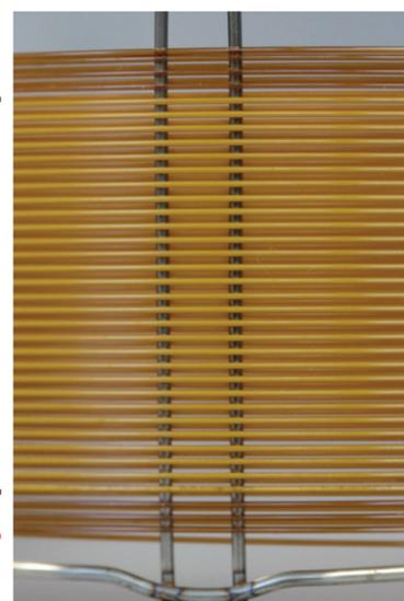
Figure 1: Integral 2.5-m particle traps at both ends of the GC column.
