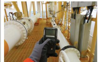
Hand-held portable gas leak detection
