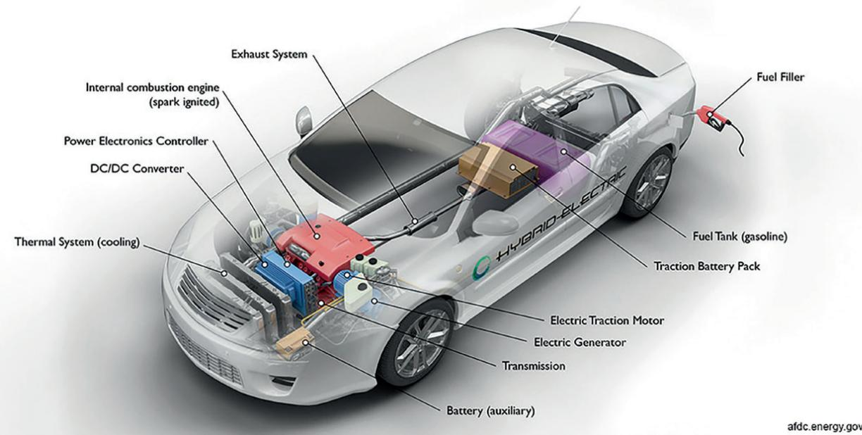
Fig. 2: Diagram of a hybrid electric vehicle, as depicted by the U.S. Department of Energy [9].
