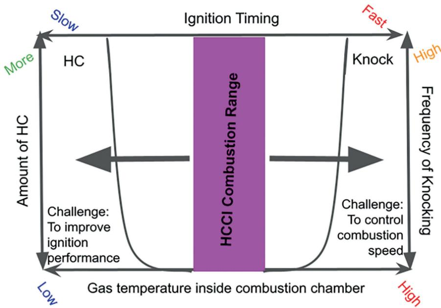
Fig. 4: Graph indicating the fine-tuned combustion range of HCCI combustion [12].
