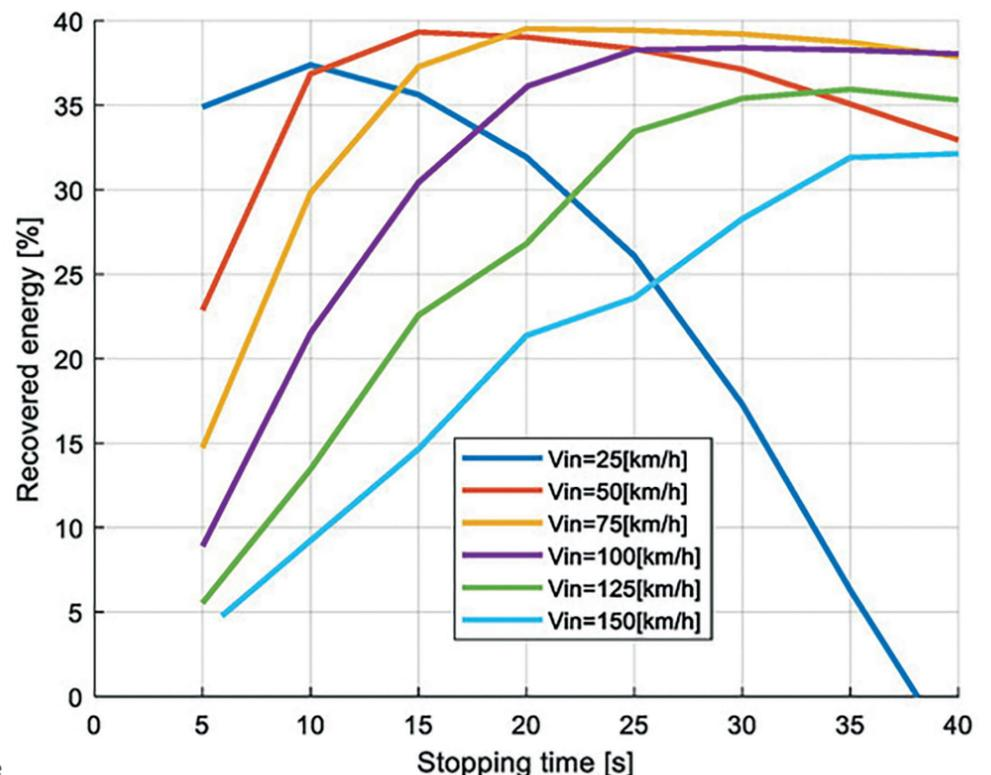
Fig. 3: Recovered energy percentage against stopping time at various speeds, as determined by Rizzo's team [10].
