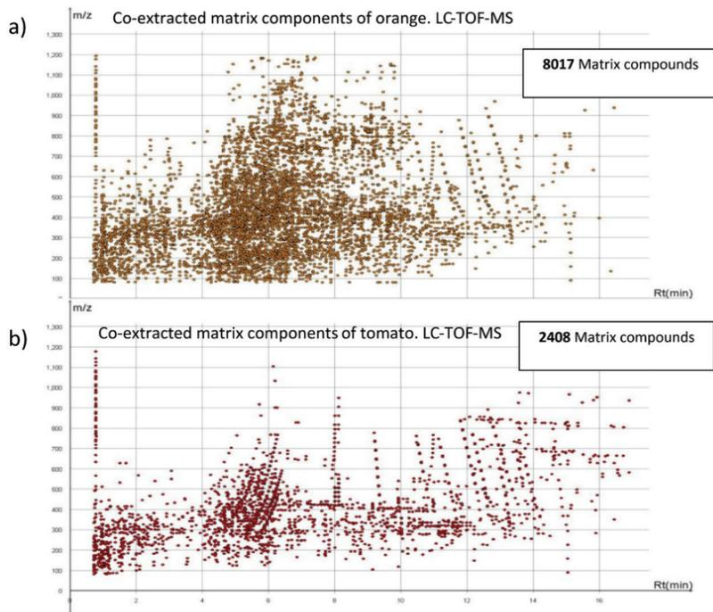
Figure 3: Matrix compounds of orange (a) and tomato (b) extracts analyzed using a 6530 Agilent LC-QTOF-MS. The HPLC system used was the 1200 series from Agilent Technologies, equipped with a XDB-C18 analytical column of 4.6 mm x 50 mm and 1.8 μm particle size
