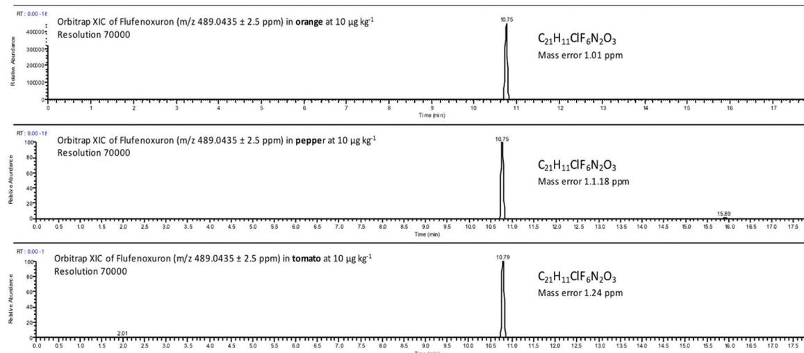
Figure 7: Detection of pesticide flufenoxuron at  $10 \mu\text{g}\cdot\text{kg}^{-1}$  in tomato, pepper and orange. Resolution 70000, mass tolerance of 5 ppm. Analyzed by Orbitrap QExactve (ThermoFisher Scientific, Bremen, Germany) mass spectrometer. The UHPLC system used for these tests was the Dionex Ultimate 3000. It was equipped with an Thermo Accucore C18 column  $150\times 2.1\text{mm}$ ;  $2.6 \mu\text{m}$  particle size held at  $25^\circ\text{C}$
