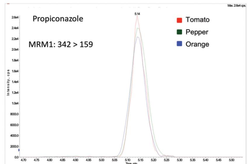
Figure 5: Propiconazole at 10 μg·kg<sup>-1</sup>, diluted 30 times, in three different matrices analyzed by a 4500 AB SCIEX QTRAP LC-MS/MS system. The HPLC system used was the Eksigent ekspert™ microLC 200, equipped with a Halo C18 column, 0.5 x 50 mm, and a 2.7 μm particle size at 30 °C (Eksigent, AB SCIEX Instruments, Foster City, CA)
