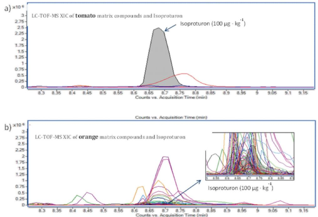
Figure 4: Extracted ion chromatogram of Isoproturon ( $m/z$  207.1492) and co-eluting matrix compounds in tomato (a) and orange (b). Analyzed by a 6530 Agilent LC-QTOF-MS. The HPLC system used was the 1200 series from Agilent Technologies, equipped with a XDB-C18 analytical column of 4.6 mm x 50 mm and a 1.8 μm particle size
