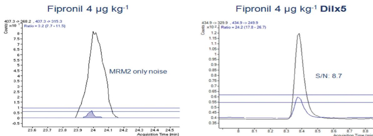
Figure 2: HPLC-MS/MS chromatograms of fipronil at  $4 \mu\text{g}\cdot\text{kg}^{-1}$  in fruit-based baby food using: a) a 6410 Agilent LC-QQQ-MS/MS system and b) a 6490 Agilent LC-QQQ-MS/MS system. The HPLC system used was the 1200 series from Agilent Technologies, equipped with an Eclipse XDB C8 analytical column of  $150\times 4.6\text{mm}$ ; and a  $5 \mu\text{m}$  particle size
