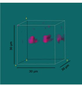
Microscopic image of a water flea (Daphnia magna) and Raman microscopic analysis of a segment (green frame in the left image) in the intestine of the animal. The magenta colored areas in the right image show PVC particles taken up by the animal. (Picture: H. Imhof and P. Anger / TUM)
