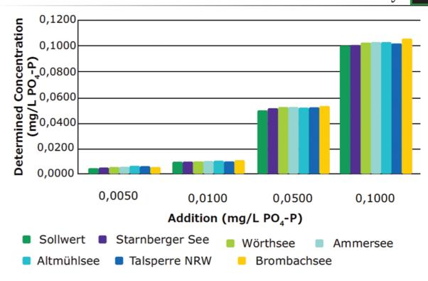
Figure 1: Orthophosphate concentration recovered after standard addition
