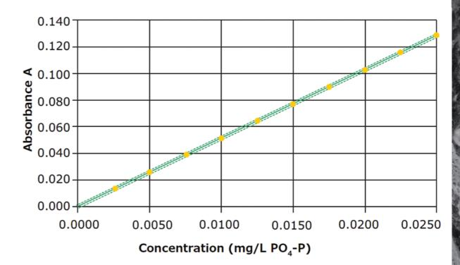
Figure 2: Calibration curve for the measurement range 0.0025 – 0.0250 mg/L PO<sub>4</sub>-P
