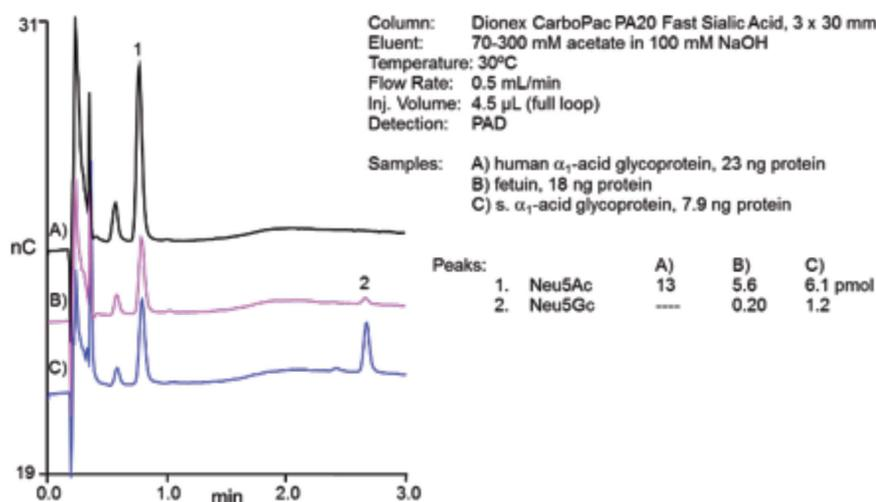
Figure 4. Fast separation of glycoprotein acid hydrolysates using HPAE-PAD
