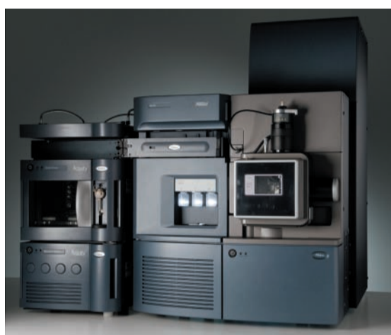
Figure 1. Xevo QToF MS with ACQUITY UPLC.
