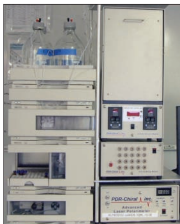
Figure 2: AutoMDS on Agilent 1100 with 22 Columns & 20 Bottles
