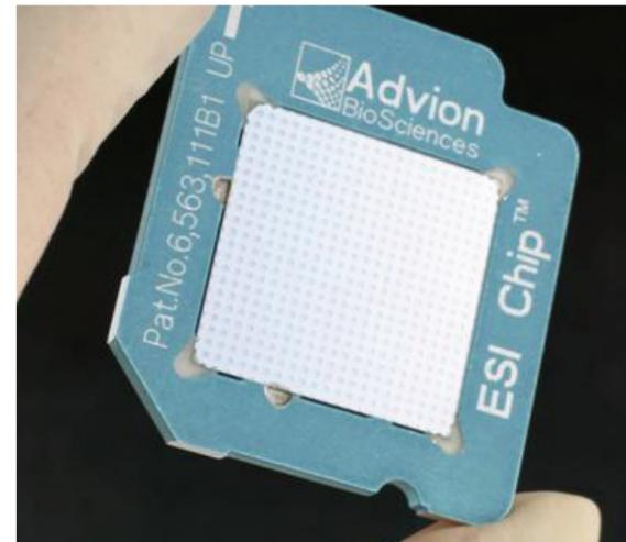
The ESI Chip: Array of 400 independent nanoelectrospray nozzles
